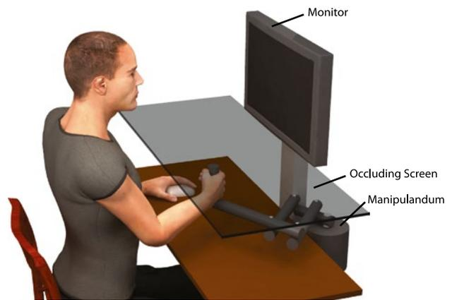
**Fig. 1** Side view of the experimental setup. In the experiment, a drape occluded view of the arm and the occluding screen was opaque. (The drape is absent and occluding screen left transparent for illustration purposes). The manipulandum presented the shapes by passively moving the unseen hand, and in secondary task conditions, *arrows* were presented on the computer monitor
